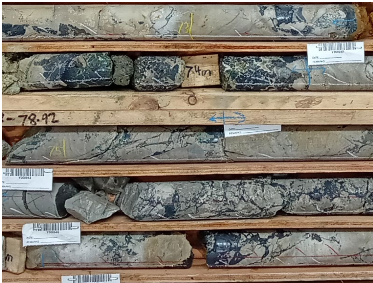
Figure 4: Dense semi-massive and breccia visual chalcocite (dark grey mineral) from PFS-002 (72.7-76.5m downhole). This interval assayed at an average grade of 8.3% Cu, 31g/t Ag.
