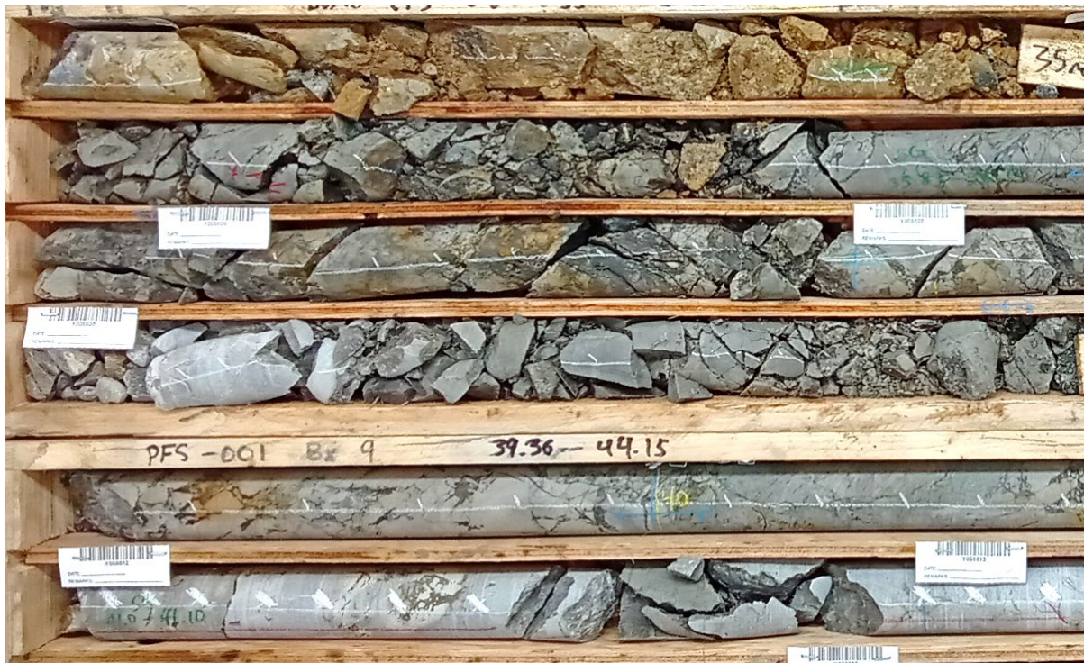
Figure 3: Dense breccia and semi-massive visual chalcocite (dark grey mineral) in drill hole PFS-001 (33.4-40.5m downhole). This interval assayed at an average grade of 2.2% Cu, 12g/t Ag.
