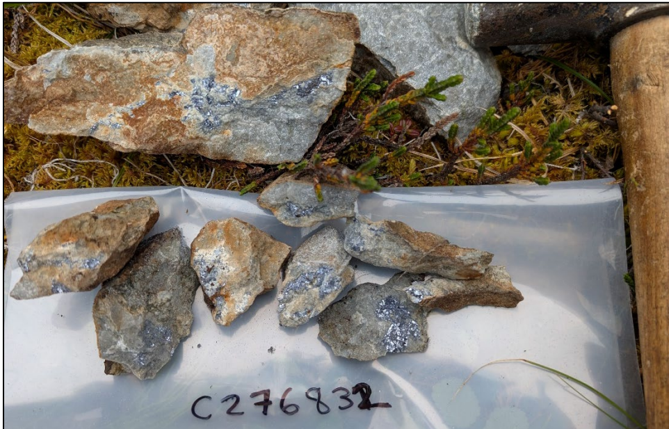
Figure 6: Galena mineralization in dolomite at Bob Showing, yielding up to 17.8% Pb and 1.9% Zn.
