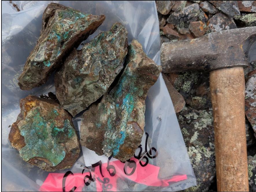
Figure 3: Disseminated chalcopyrite-bornite at the Expert Showing, yielding up to 5.42% Cu and 1.89 g/t Au. Chalcopyrite is the yellow metallic mineral, with bornite (purple-blue), with surficial recent weathering to green malachite.
