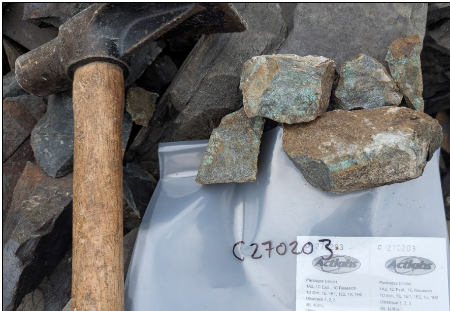
Figure 4: Quartzite boulders with disseminated chalcopyrite-bornite at the Clastic Showing, up to 3.7% Cu and 2.08 g/t Au.
