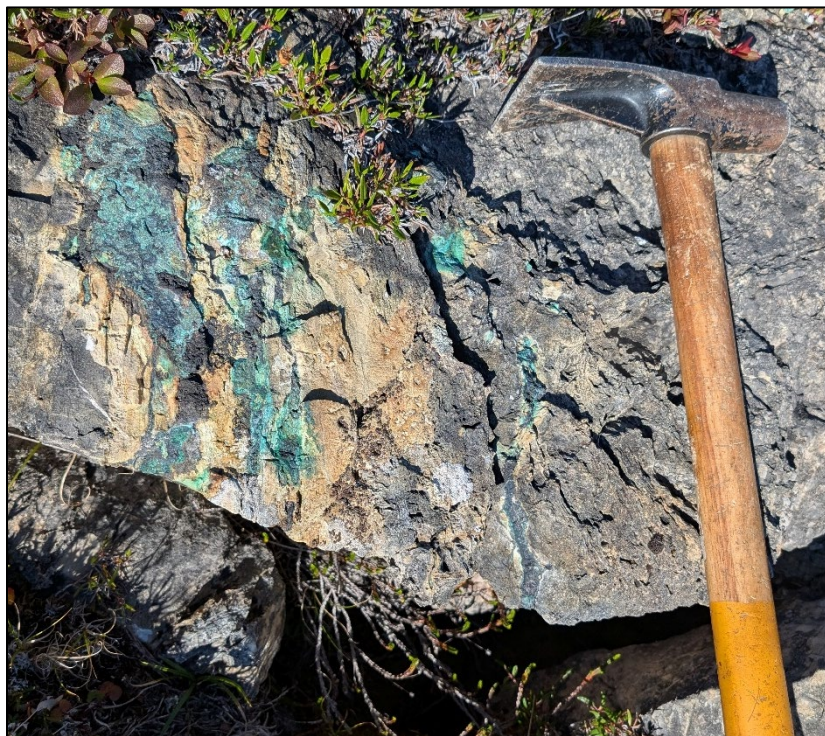
Figure 2: Chalcocite veinlets in dolomite at the Greenback Showing, yielding up to 29.2% Cu with 217 g/t Ag. Chalcocite is the dark grey metallic mineral that shows minor surficial weathering to green malachite.
